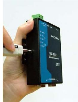
**Step 2:** Remove the UC-7112-LX Plus's outer cover.
